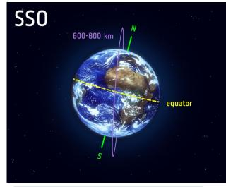
A sun-synchronous orbit (SSO) is a special type of low-Earth orbit (LEO) (Source: ESA)
