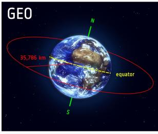
A geosynchronous equatorial orbit (GEO) (Source: ESA)
