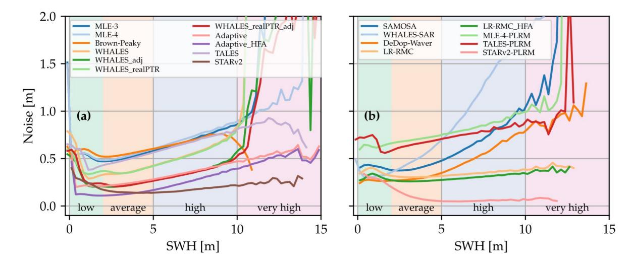
Figure 2. Noise level of the individual retrackers as a function of significant wave height (SWH) for (a) J3- and (b) S3A-retracking algorithms with the sea state noted at the bottom.
