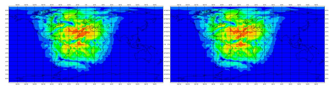
Surface downward solar radiation for the original scheme and the neural network emulator (based on a ResNet).
