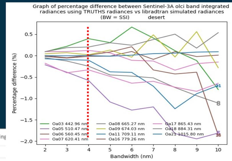
TRUTHS' spectral BW < specification. Mostly 2-3 nm in Vis and 5-6 nm in SWIR
