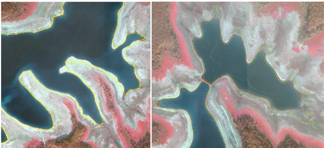
Figure 36: Comparison of VHR/HR in Orient Lake Red lines are the LWE limits derived from Pleiades NEO, yellow lines the Sentinel LWE limits
