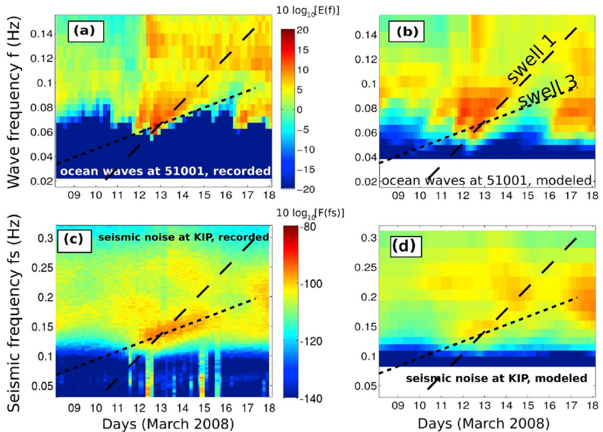
Figure 2: Example of seismic spectrogram (bottom) observed and modeled, compared to wave spectra (top). Taken from Ardhuin et al. (2011).
